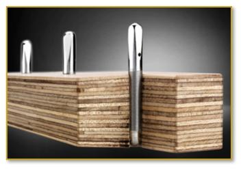
quarter sawn hard-rock maple which is cross laminated to ensure maximum resistance on the tuning pin threads. Tuning pins are nickel plated to resist rust and insure string integrity.
